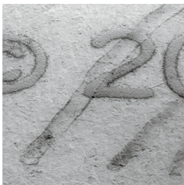
Figure 8. Low voltage imaging showing ink on top of printed letter
